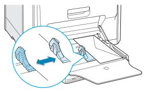
5 When you print, configure the paper source to **MP Tray**, the paper type to **Envelope** and the paper size in the software application. For details, see page 4.7.
